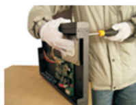
1. Install fixed screw for HDD
